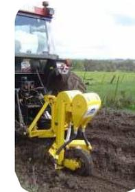
At the rear of the tractor, the Rippa Seeder scalps away topsoil, grass roots and pasture seed, leaving a shallow rip line.
